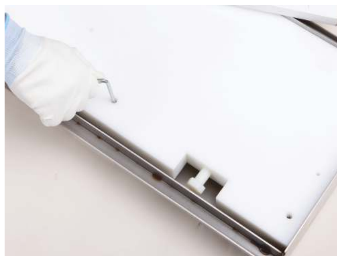
base board adjusted from its top, easier operation
